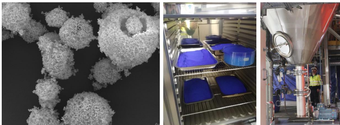
Figure 1: MOFs (HKUST-1) beads of 80 \mu\text{m} in diameter prepared by spray-drying process
